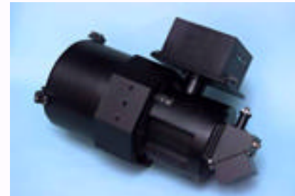
Optical Comm Demonstrator - 10 cm telescope - Fiber-coupled laser
