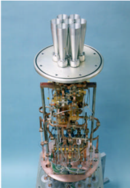
Seven Element Array Feed with 4.45-cm Diameter Dual-Mode Horns
